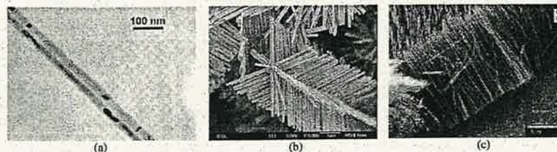
Figure 1.4 Examples of nanowires and nanotubes synthesized by various methods: (a) a pair of bismuth nanowires obtained by pressure injection into a template (Dresselhaus et al., 2001; courtesy of Dr. M.S. Dresselhaus), (b) \text{TiO}_2 nanowires obtained by vapor condensation (courtesy of Dr. Z.F. Ren), (c) carbon nanotubes grown by plasma CVD (Ren et al., 1998; courtesy of AAAS).
